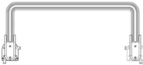
Drapery Track with a 45° Double Bend
