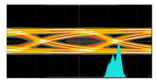
Figure 6. 3840×2160 30 fps video, results as seen at the sink (display device) end of a 3-foot HDMI cable.
