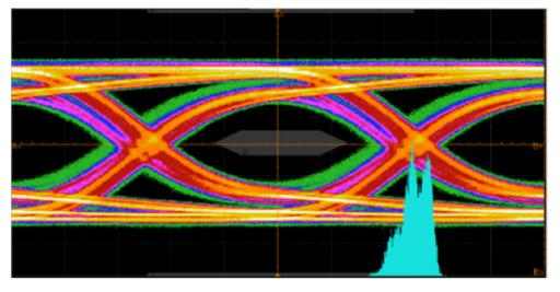
Figure 5. 1920×1080 60 fps video, results as seen at the sink (display device) end of a 3-foot HDMI cable.
