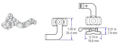
Cam Lock Mounting Bracket (Qty. 2) (CSA-DRP-CAM-LOCK)
