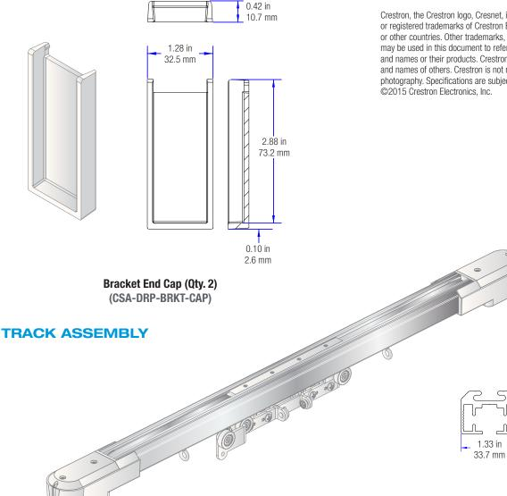
Drapery Track Assembly (Shown with Splice Bar) (CSA-DRP-TRACK-ASM)
